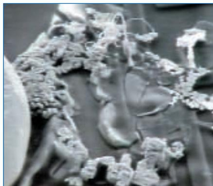
Figure 5. Dendrite growth in sidebrazed packaging Experiment 2.
