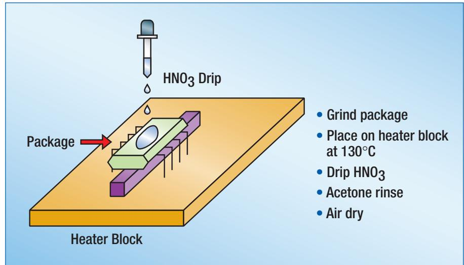
Figure 1. Standard decapsulation process
