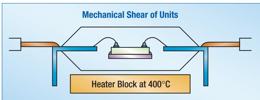
Figure 4. Mechanical shear of units from Experiment 3
