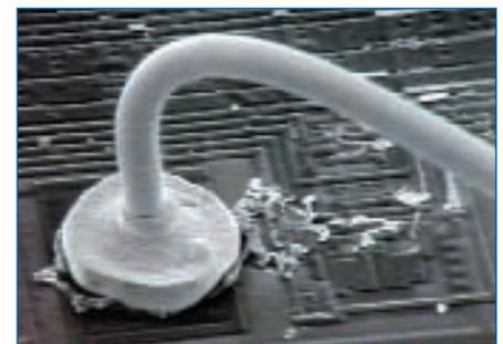
Figure 2. Photo of SEM studies showing the presence of silver dendrites after the decap.
